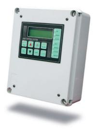
The remote control unit (REM) is an electronic card that communicates with the Q500 rectifier, up to 100 meters away, via serial communications (through CRS-ASCII or Modbus-RTU protocol) or analogue control.
